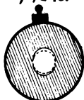
The wearing away of the bore caused by cleaning from the muzzle end with a metal rod.
